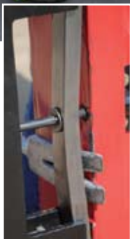
Above: The Inforcer lets you practice sound forcible entry techniques before you need to use them on an inward-swinging door on the fireground.
